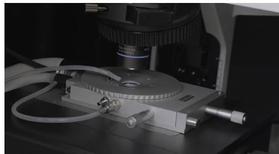
Figure 1. An n -doped Si wafer inside a Linkam THM600, fitted to an RM5
