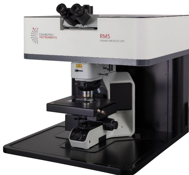
Figure 3. The RM5 Raman Microscope
